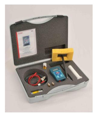
The Buckleys LVPD utilises the wet sponge and provides a quick and cost effective method of non-destructively testing dielectric coatings on conductive substrates up to 500µm.
